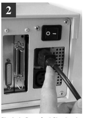
Plug in the Power Cord. Plug the other end into a power socket.
